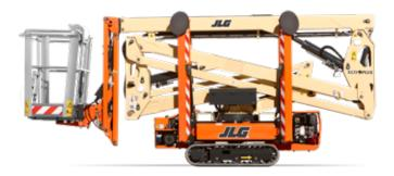
With outrigger pads removed. Pads increase width by 196 mm and height by 124 mm in stowed position.
